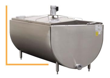
Open type semi cylindrical rectangular shaped direct expansion cooling tank. It has opening lids for easy access and rounded internal corners to facilitate through cleaning. Tank insulation is provided by factory injected pollyurethane foam of 50mm. The integral condensing unit is Hermetic type with R22 refrigerant. The condensing unit is beneath the tank of occupy minimum space.
