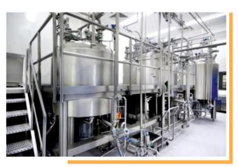
Oral liquid manufacturing plant comprises of sugar syrup vessel, online sugar syrup pre-filter, manufacturing vessel storage vessel, vacuum system for transfer of sugar and sugar syrup, product piping, control panels and transfer pumps. The construction of the complete system is done in a way that allows for plant to be easily handled by single operator, thus saving on man-power costs. Further, the system also comes with limpet coils for desired heating and cooling
