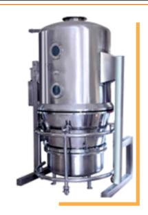
We offer Fluid Bed Dryers that contains no moving part inside the drying chamber where the different operations take place for the drying of the material. These machines incorporate phenomenon of fluidisation, for production of full agitation of solid particles by hot and uniform air. The salt is fluidized, each particle meets the hot air, discharges moisture and dries at the same time traveling forward without any mechanical push.
